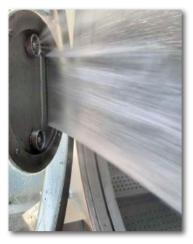
Due to the special design of the dyeing system sprays the chemicals on the cover into the drum. It reduces the liquor ratio to 1:2, 1:3.
